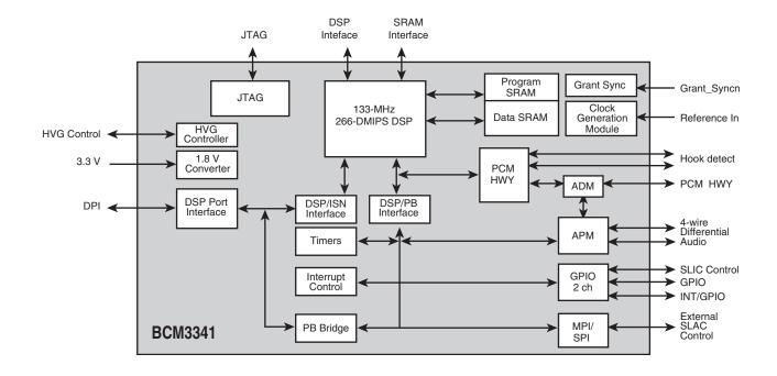
The BCM3341 offers the industry a highly integrated, cost effective approach to developing voice cable modem solutions for the delivery of primary or secondary line telephony. The BCM3341 provides a seamless interface to the BCM3349 single chip DOCSIS/EuroDOCSIS<sup>TM</sup> 2.0 cable modem.
