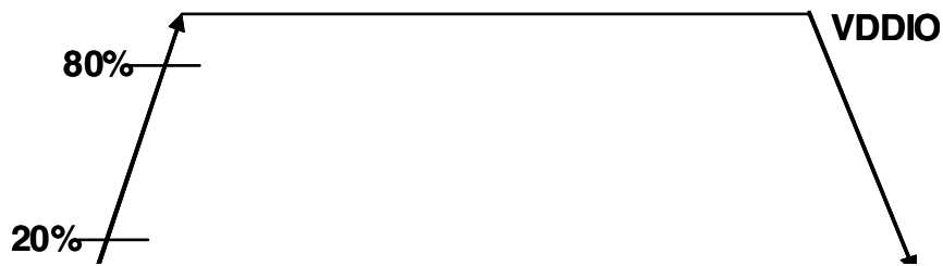
Figure 4. Output Pad Transition Waveform
