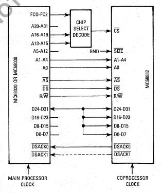
Figure 13. 8-Bit Data Bus Coprocessor Connection
