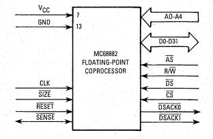
Figure 10. MC68882 Input/Output Signals
