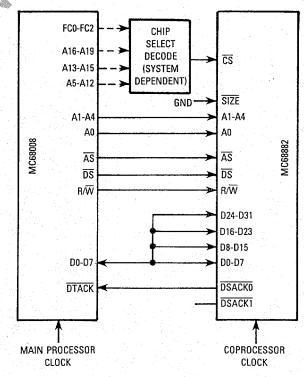
Figure 15. 8-Bit Data Bus Peripheral Processor Connection
