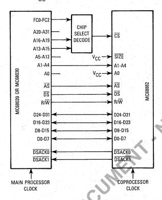
Figure 11. 32-Bit Data Bus Coprocessor Connection
