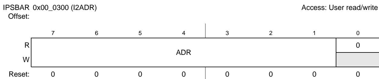
Figure 24-2. I 2 C Address Register (I2ADR)
