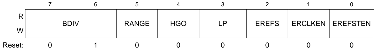
Figure 11-4. ICS Control Register 2 (ICSC2)
