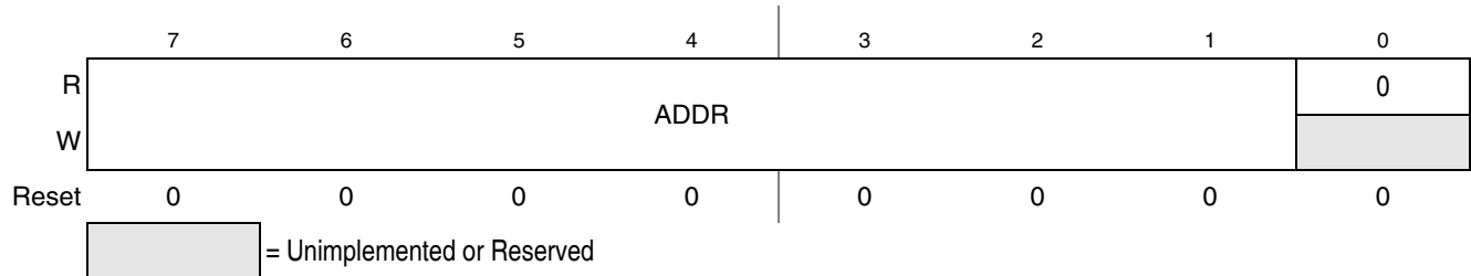
Figure 11-3. IIC Address Register (IICA)
