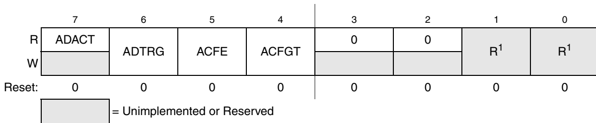
Figure 9-5. Status and Control Register 2 (ADCSC2)
