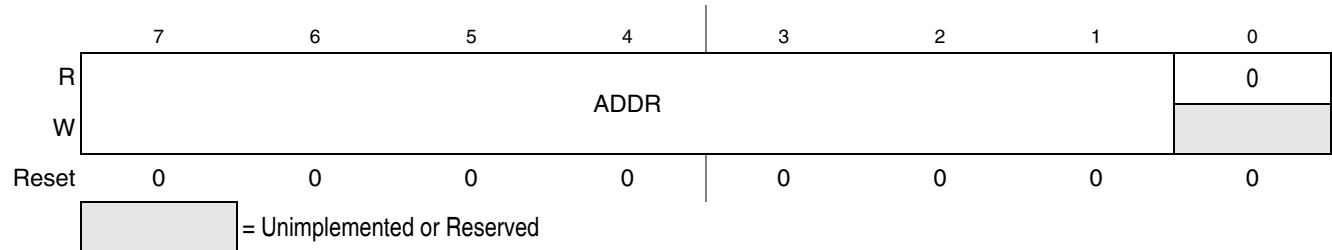
Figure 11-3. IIC Address Register (IICA)
