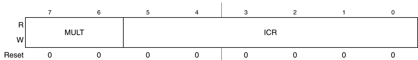
Figure 11-4. IIC Frequency Divider Register (IICF)
