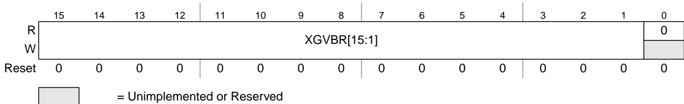
Figure 6-5. XGATE Vector Base Address Register (XGVBR)
