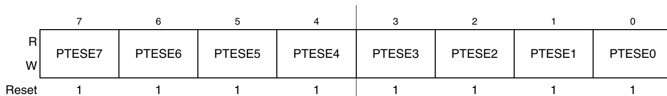
Figure 6-25. Output Slew Rate Control Enable for Port E (PTESE)
