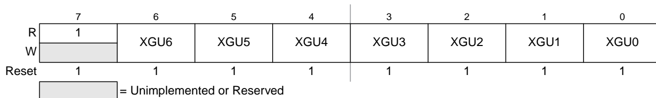
Figure 18-18. RAM XGATE Upper Boundary Register (RAMXGU)
