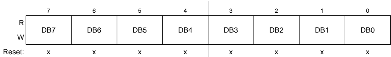
Figure 10-34. Data Segment Registers (DSR0–DSR7) — Extended Identifier Mapping
