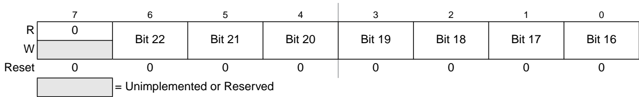
Figure 20-15. Debug Comparator Address High Register (DBGXAH)
