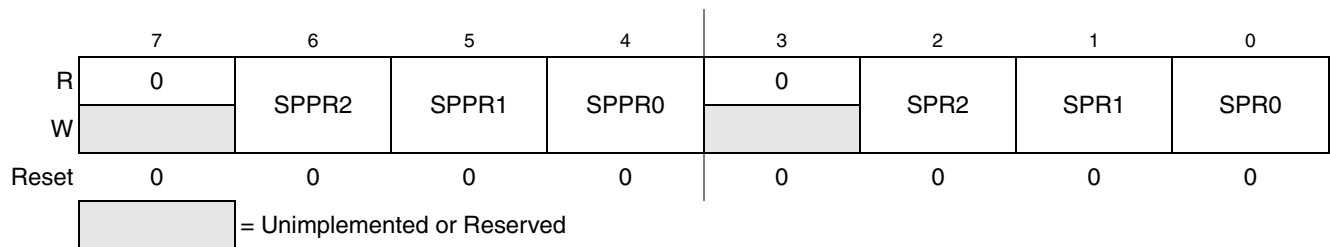
Figure 12-7. SPI Baud Rate Register (SPI1BR)
