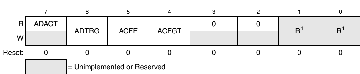
Figure 9-5. Status and Control Register 2 (ADCSC2)
