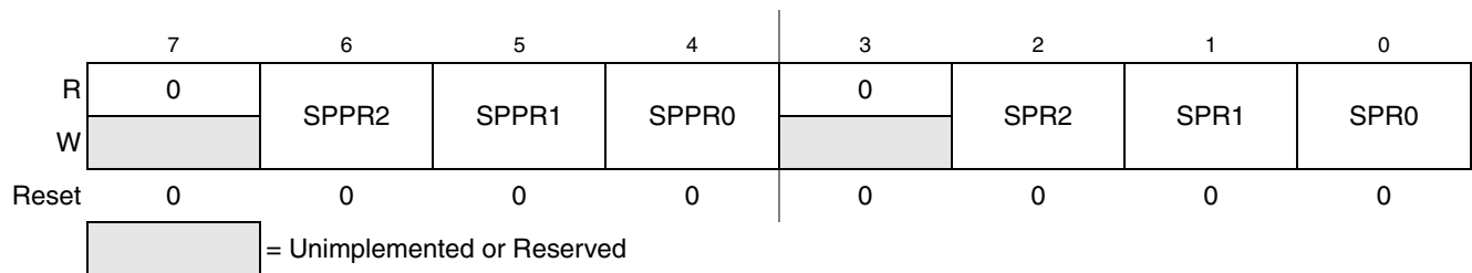
Figure 15-7. SPI Baud Rate Register (SPIBR)
