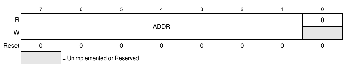
Figure 13-3. IIC Address Register (IIC1A)
