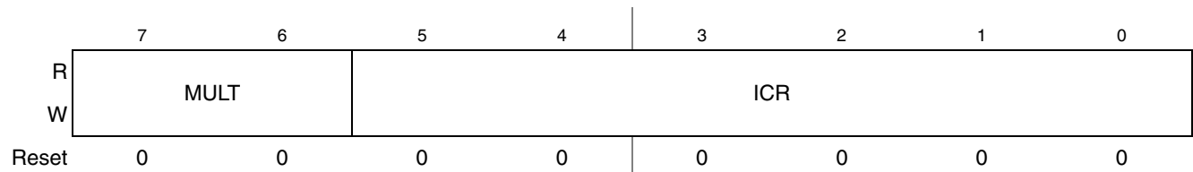
Figure 13-4. IIC Frequency Divider Register (IIC1F)
