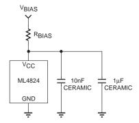
Figure 3. External Component Connections to VCC
