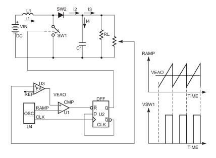
Figure 5. Typical Leading Edge Control Scheme.
