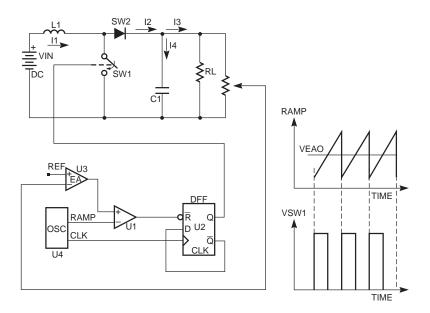
Figure 4. Typical Trailing Edge Control Scheme.
