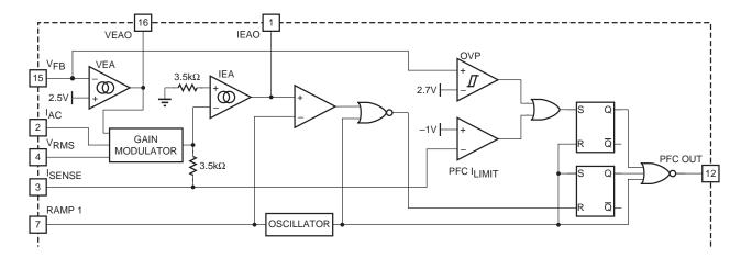
Figure 1. PFC Section Block Diagram.
