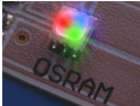
By using 3 diodes in one LED package, color mixing is achieved without color separation.
