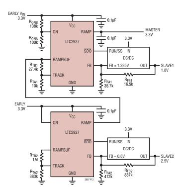
Figure 12. Ratiometric Tracking Example
