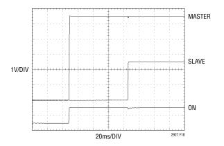
Figure 18. Power Supply Start-Up Delayed
