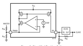
Figure 5. Simplified Tracking Cell
