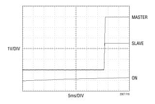
Figure 19. ON Pin Delayed
