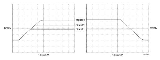
Figure 9. Coincident Tracking (from Figure 10)
