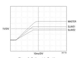
Figure 3. Ratiometric Tracking
