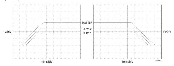
Figure 13. Offset Tracking (from Figure 14)
