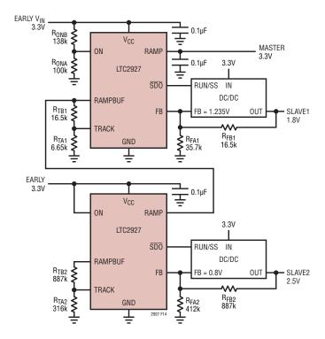
Figure 14. Offset Tracking Example
