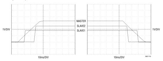
Figure 15. Supply Sequencing (from Figure 16)
