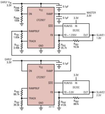
Figure 16. Supply Sequencing Example
