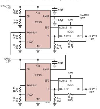
Figure 10. Coincident Tracking Example
