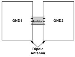
Figure 15. Dipole Antenna
