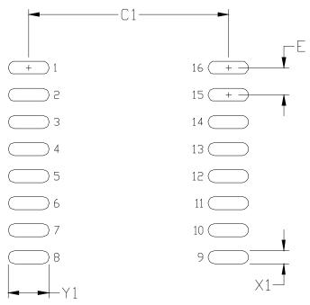
Figure 18. 16-Pin SOIC Land Pattern
