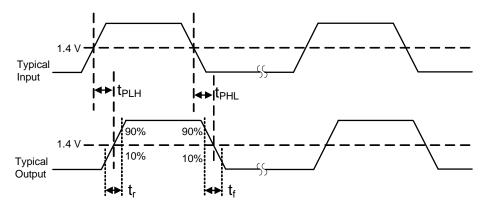
Figure 2. Propagation Delay Timing
