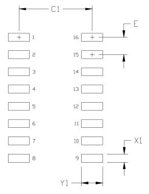
Figure 20. 16-Pin Narrow Body SOIC PCB Landing Pattern
