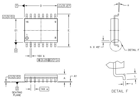
Figure 17. 16-Pin Wide Body SOIC
