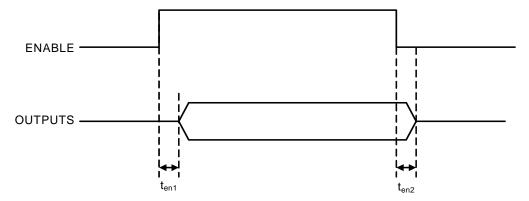
Figure 1. ENABLE Timing Diagram
