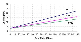
Figure 6. Si8441 Typical V<sub>DD1</sub> Supply Current vs. Data Rate 5, 3.3, and 2.70 V Operation
