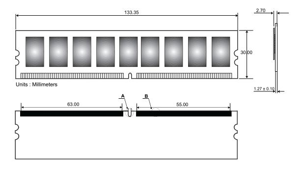
Figure 1: KVR400D2E3/1G 240-Pin DIMM
