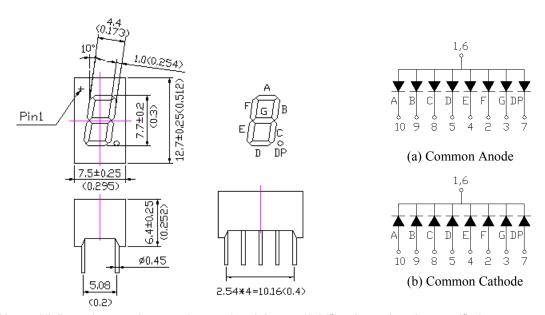
Notes: All dimensions are in mm, tolerance is  $\pm$  0.25 mm (0.01") unless otherwise specified
