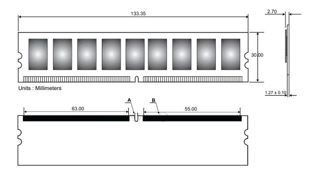
Figure 1: KVR800D2E5/1G 240-Pin DIMM
