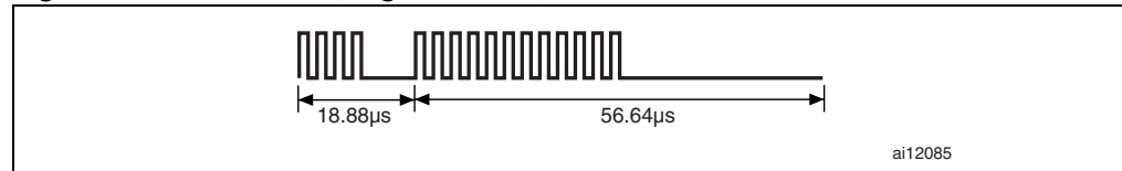
Figure 31. End of frame, high data rate, one subcarrier x2
