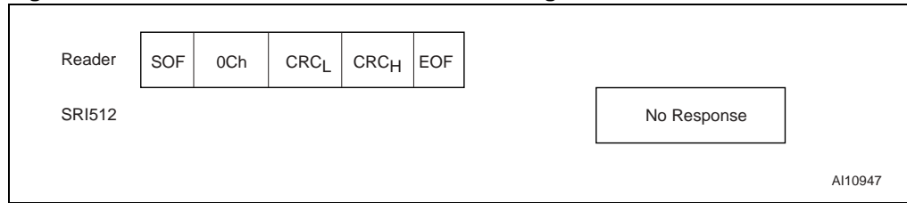
Figure 61. READ_BLOCK frame exchange between Reader and SRI512
