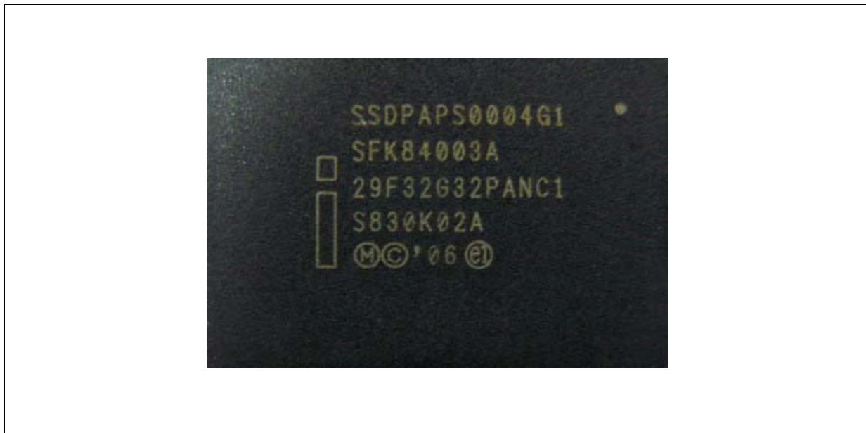
Figure 1. Front View of the Intel Z-P140 PATA SSD
