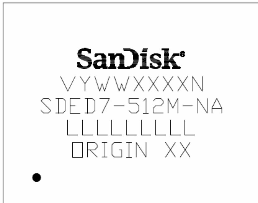
Figure 40: Example of SDED7-512M-NA Product Marking
