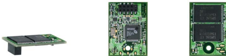
Figure 4: uDiskOnChip Horizontal Version with Single Connector
