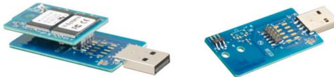
Figure 10: uDiskOnChip External USB Adapter, with and without Mounted Device
