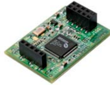
Figure 5: uDiskOnChip Horizontal Version with Dual Connector Configuration
