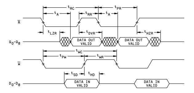
FIGURE 3. Timing waveforms.
