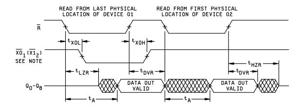
NOTE: Expansion out of device 1 (XO<sub>1</sub>) is connected to expansion in of device 2 ( $\overline{XI}_2$ ).
