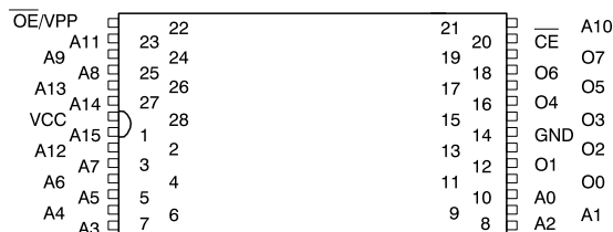
TSOP Top View Type 1
