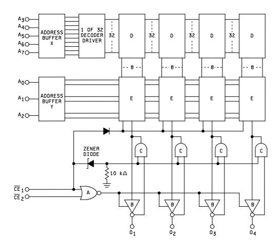
A = Enable buffer B = Output buffer
