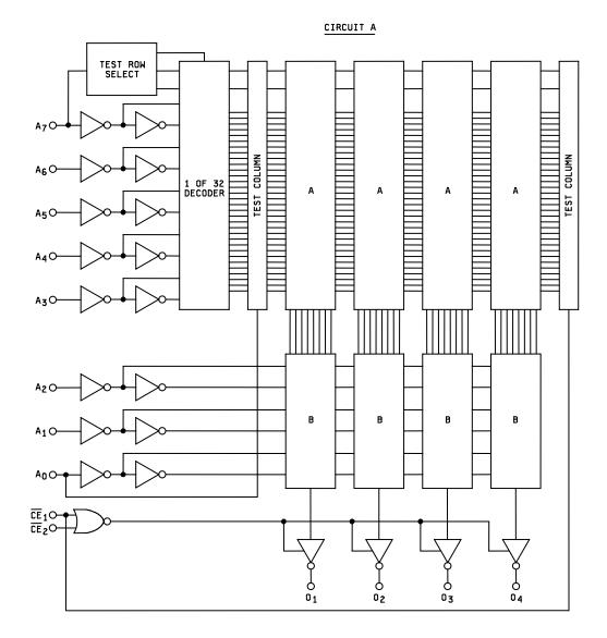
$A = 32 \times 8$  Memory Array B = 1 of 8 Decoder
