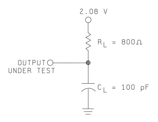
FIGURE 4. Output load circuit.
