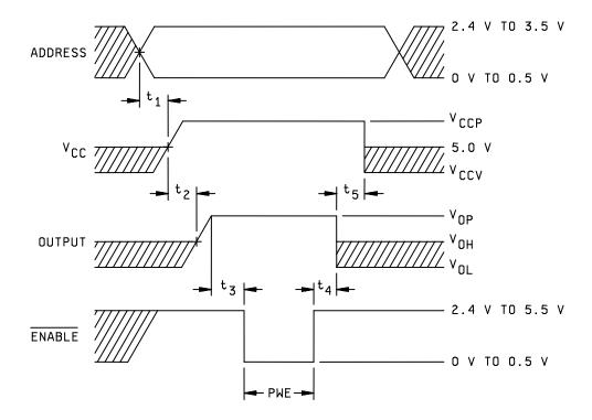
FIGURE 5D. Typical programming voltage waveforms during programming for circuit G.
