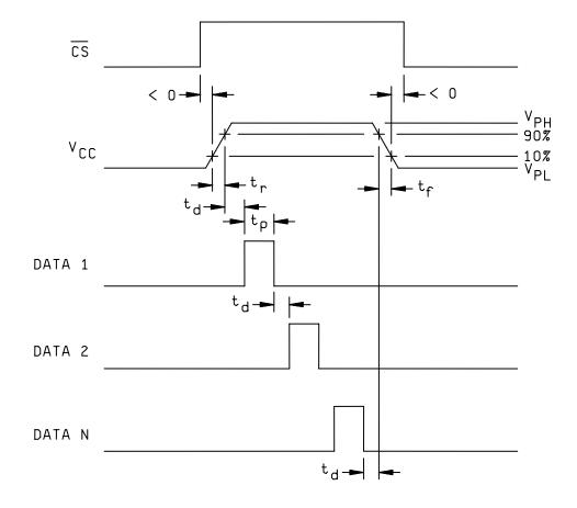
FIGURE 5J. Programming voltage waveforms during programming for circuit J.
