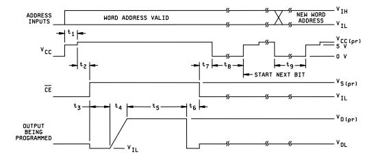
FIGURE 5H. Programming voltage waveforms during programming for circuit H.
