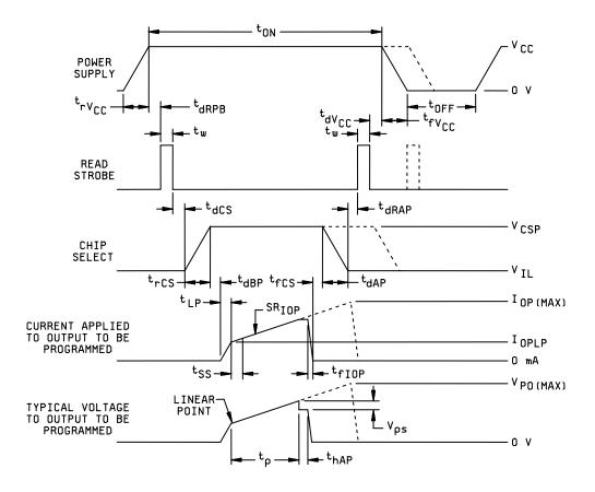
FIGURE 5D. Programming voltage waveforms during programming for circuit D.
