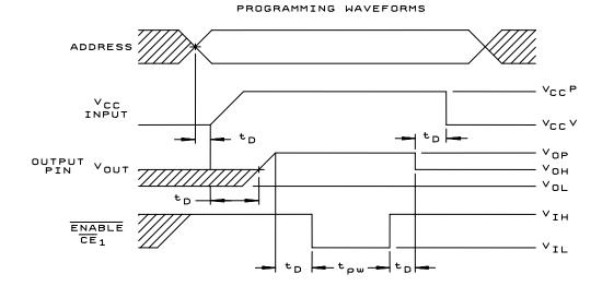
FIGURE 5B. Programming voltage waveforms during programming for circuit B.
