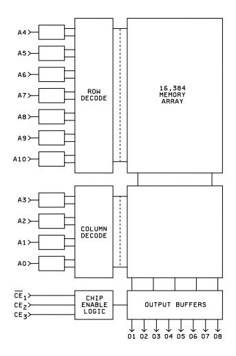
FIGURE 3. Functional block diagrams.
