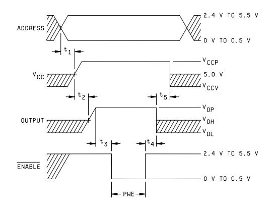
FIGURE 5G. Programming voltage waveforms during programming for circuit G.
