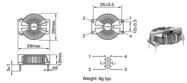
Recommended hole diameter: ød+0.5 Dimensions in mm
