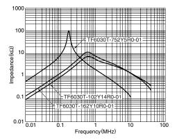
Common Mode Choke Coils(Line Filters) for AC Power Supply Toroidal Core Type for 3-Phase
