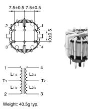
Recommended hole diameter: ø1.3 Dimensions in mm
