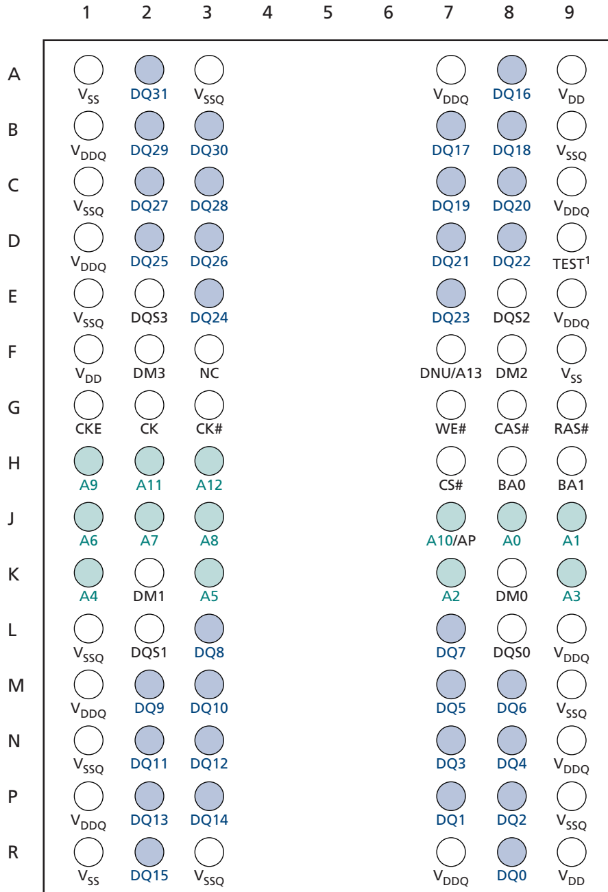
Figure 5: 90-Ball VFBGA – 10mm x 13mm and 9mm x 13mm (Top View)
