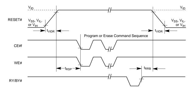
Figure 25. Temporary Sector/Sector Block Unprotect Timing Diagram
