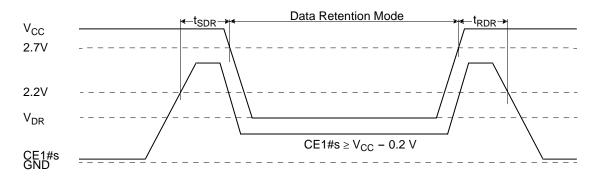
Figure 33. CE1#s Controlled Data Retention Mode
