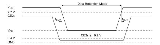
Figure 34. CE2s Controlled Data Retention Mode
