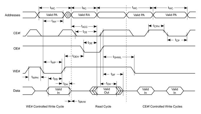
Figure 21. Back-to-back Read/Write Cycle Timings
