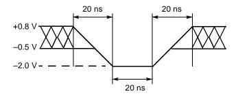
Figure 7. Maximum Negative Overshoot Waveform
