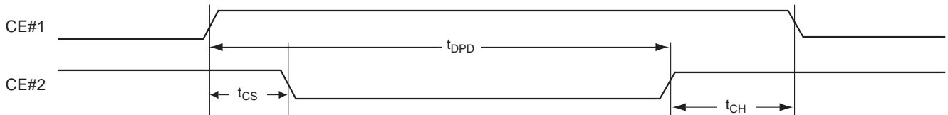
Figure 32. Deep Power-down Timing
