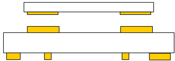
Figure 20. Correct PCB Top Metal Pattern Under Package
