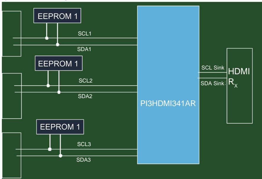
This architecture allows EDID readability when the DTV is power off or power on.
