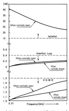
When normally closed: MS-135 single item condition When normally open: MS-135 and MS-135-C (P) coupled condition
