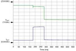
Kickstart Response Normal Load with Temporary Short Circuit
