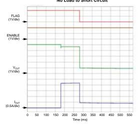
Kickstart Response Device Enabled into a Short Circuit
