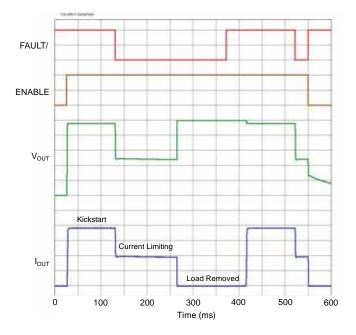
Figure 9. Kickstart operation with varying load
