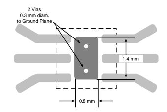
Figure 11. Pad for thermal mounting to PCB
