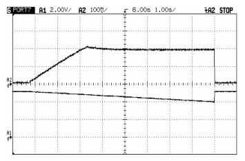
2009B SOT 502 #1 - Vout ramp 5V to 4V (5V) Radj=249ohms, Rfault=499ohms A1: Vout (2V/div) A2: lout (500mA/div)
