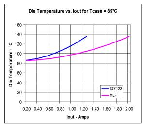
Figure 10. Die temperature vs. Package
