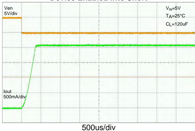
Short Circuit Current, Device Enabled Into Short
