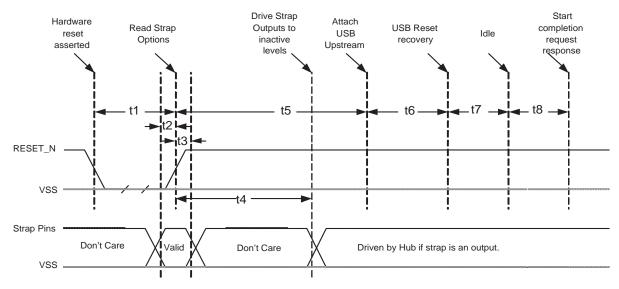
Figure 5.2 Reset\_N Timing for Default/Strap Option Mode
