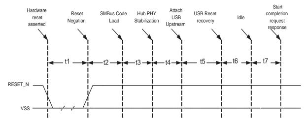
Figure 5.4 Reset\_N Timing for SMBus Mode
