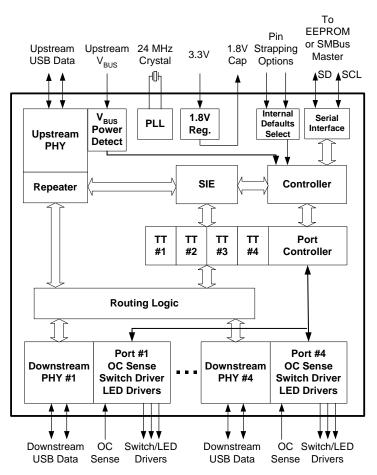
Figure 4.1 4-Port Block Diagram
