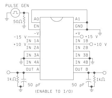
ENABLE DRIVE  $V_{AH} = 4.0 \text{ V}$  for device type 03
