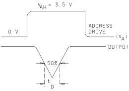
FIGURE 3. <u>Break-before-make test circuit and waveforms</u> – continued.
