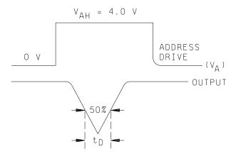
FIGURE 3. <u>Break-before-make test circuit and waveforms</u> – continued.
