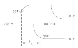
FIGURE 4. Switching times test circuits – continued.
