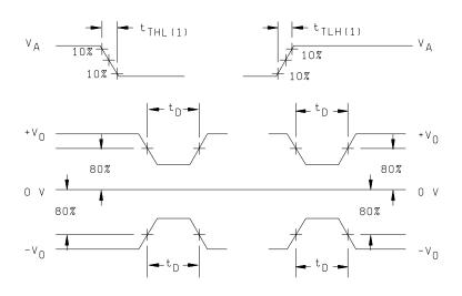
FIGURE 3. <u>Break-before-make test circuit and waveforms</u> – continued.
