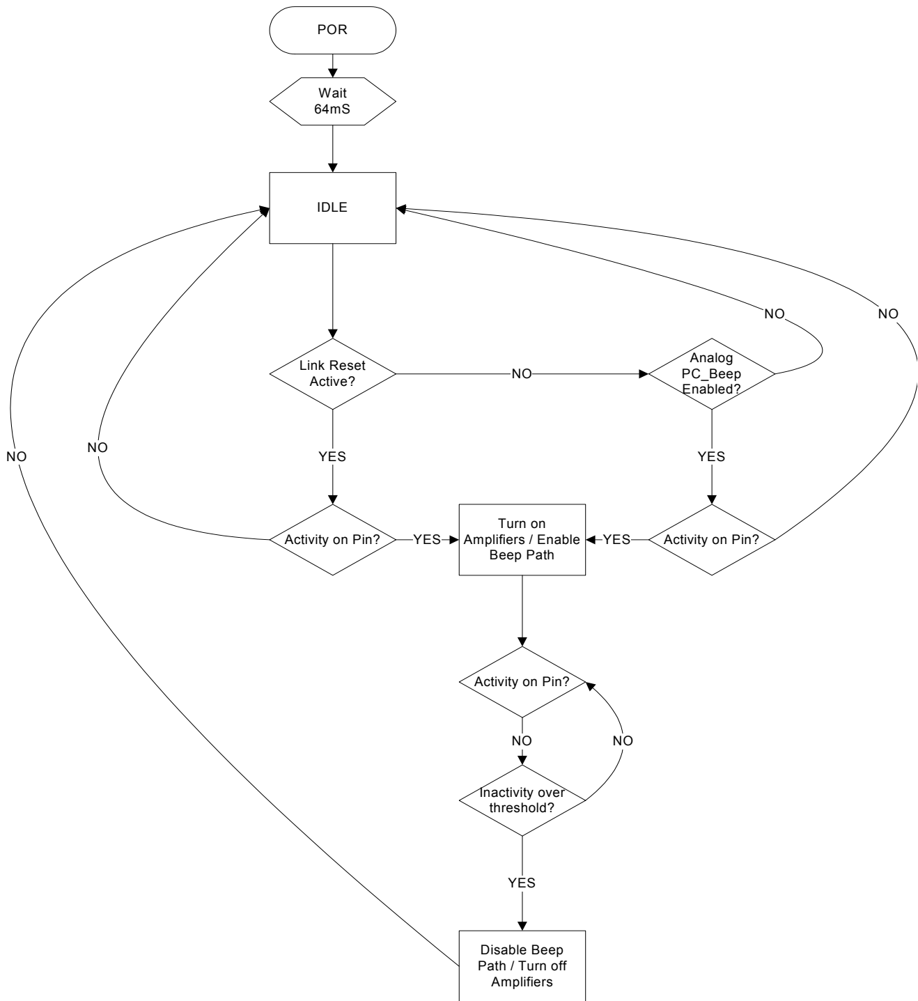
Figure 8. Analog PC Beep Flow chart
