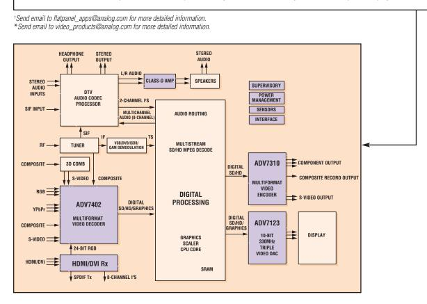
The ADV7402 and ADV7400 multiformat video decoders simplify front end digitizer and decoder architectures by reducing board space, simplifying auto detection and switching of inputs, and reducing overall system power consumption.
