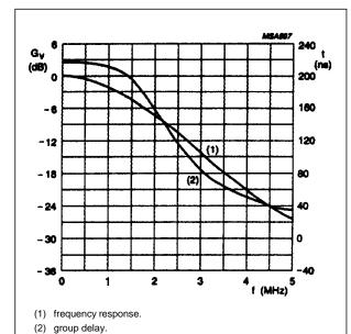
Fig.3 Low pass filter response for colour difference signals (PAL mode).
