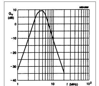
Fig.5 Band pass filter nominal frequency response (PAL mode).
