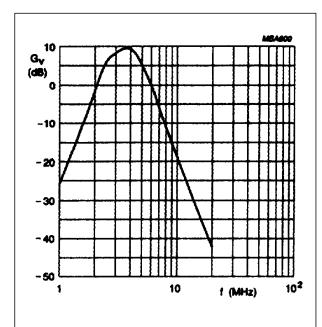
Fig.7 Band pass filter nominal frequency response (NTSC mode).
