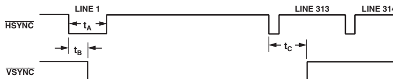
Figure 20. Timing Register 1 in PAL Mode
