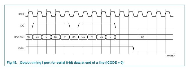
Multistandard video decoder with adaptive comb filter
