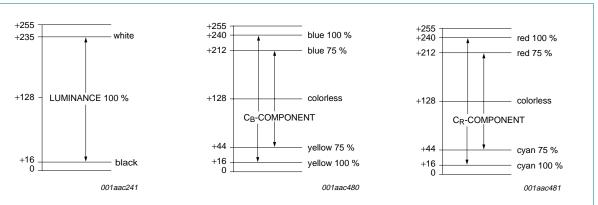
"ITU Recommendation 601/656" digital levels with default CBCS (decoder) settings CCON[7:0] = 44h, CBRI[7:0] = 80h and CSAT[7:0] = 40h.
