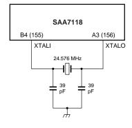
e. With fundamental quartz. Crystal load = 20 pF.
