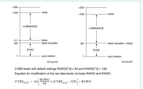
It should be noted that the resulting levels are limited to 1 to 254 in accordance with "ITU Recommendation 601/656".
