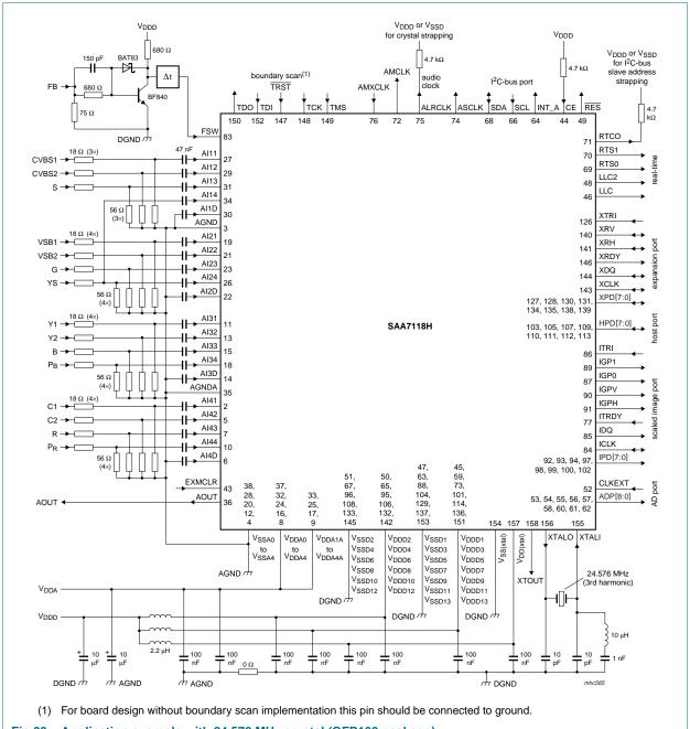
Fig 93. Application example with 24.576 MHz crystal (QFP160 package)
