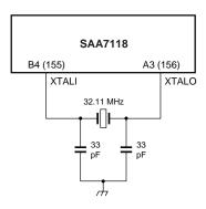
b. With fundamental quartz.Crystal load = 20 pF.
