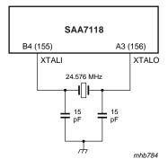
f. With fundamental quartz.Crystal load = 8 pF.
