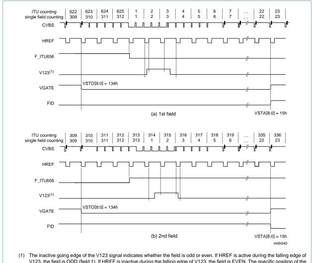
V123, the field is ODD (field 1). If HREF is inactive during the falling edge of V123, the field is EVEN. The specific position of the slope is dependent on the internal processing delay and may change a few clock cycles from version to version.
