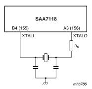
h. With fundamental quartz and restricted drive level. When P<sub>drive</sub> of the internal oscillator is too high a resistance R<sub>s</sub> can be placed in series with the output of the oscillator XTALO.
