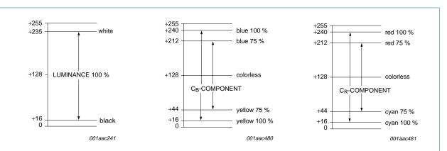
"ITU Recommendation 601/656" digital levels with default BCS (decoder) settings DCON[7:0] = 44h, DBRI[7:0] = 80h and DSAT[7:0] = 40h.
