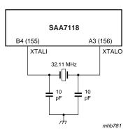
c. With fundamental quartz. Crystal load = 8 pF.
